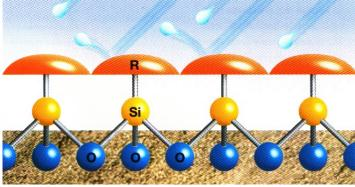
Siloseal chemically bonds to mineral surfaces forming a hydrophobic barrier.
