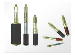
**CRG high pressure injection packers** can be used with either epoxy or polyurethane injection resins and have a maximum operating pressure of 500kgf. Packers come in standard sizes or hole diameters of 6mm to 13mm. Custom diameters and lengths can be supplied upon request.
